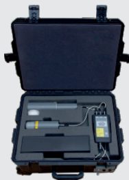
Gamma radiation and neutron radiation monitor: BDKG-11M (1 unit), BDKG-04 (1 unit), BDNG-05 (1 unit)
