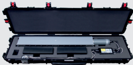
Highly-sensitive gamma radiation and neutron radiation counting monitor: BDRM-05 (1 unit), BDKN-05 (2 units)
